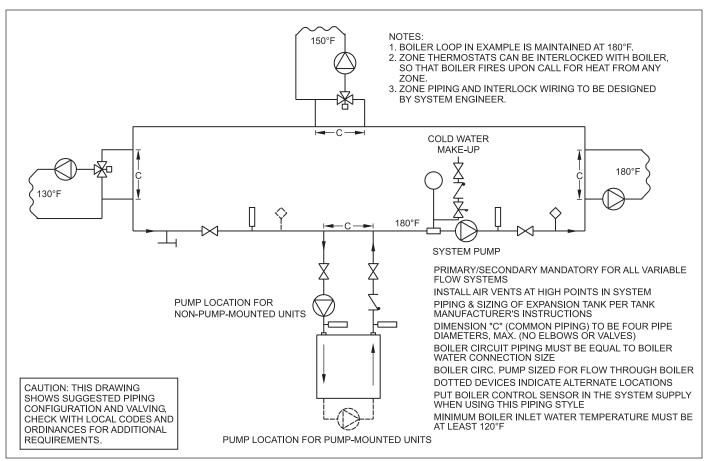
Figure 8. Hydronic Piping — One Boiler, Multi-Temperature System.
